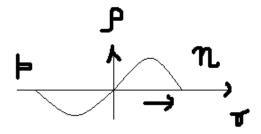
The charge density near the p-n junction (in the depletion region ) Varies with distance(r)
