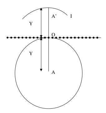
Treat A to be the spherical source of light. After time t, the wave front reach A' as wave front I. The image will be formed at A' represented by II. OA'=OA.
